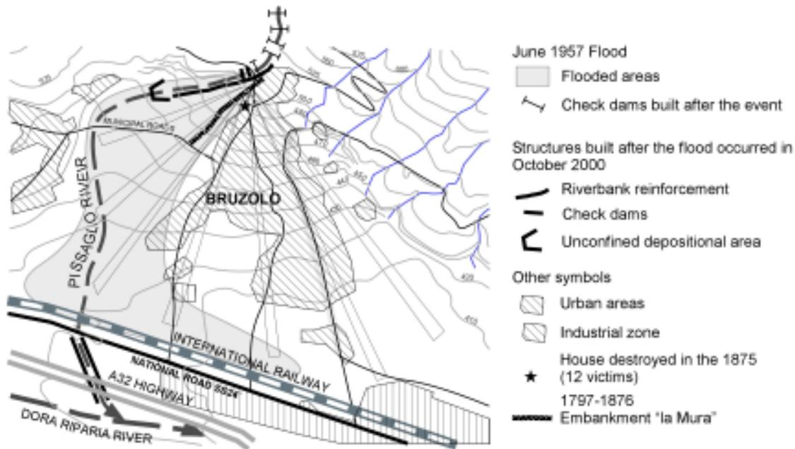
Figure 3. Maps showing the areas affected by June 1957 and October 2000 floods. River engineering structures built after these events are also displayed.
