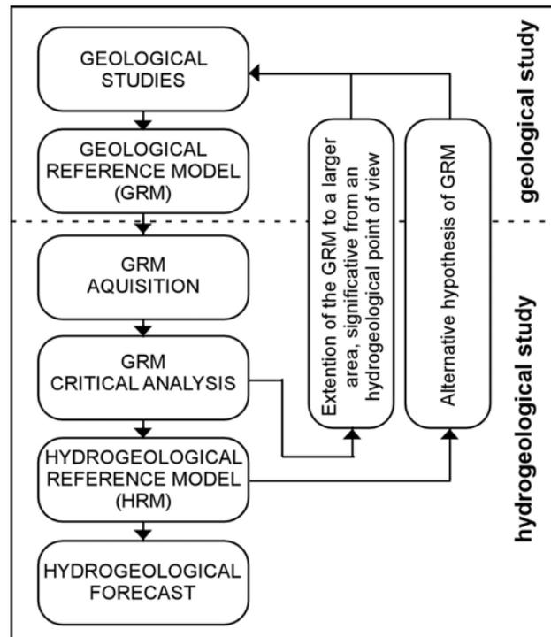
Fig. 1. Flow chart of geological and hydrogeological studies applied to deep tunnels.
