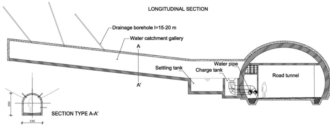
Fig. 3. Example of a water catchment gallery departing from an existing road tunnel.
