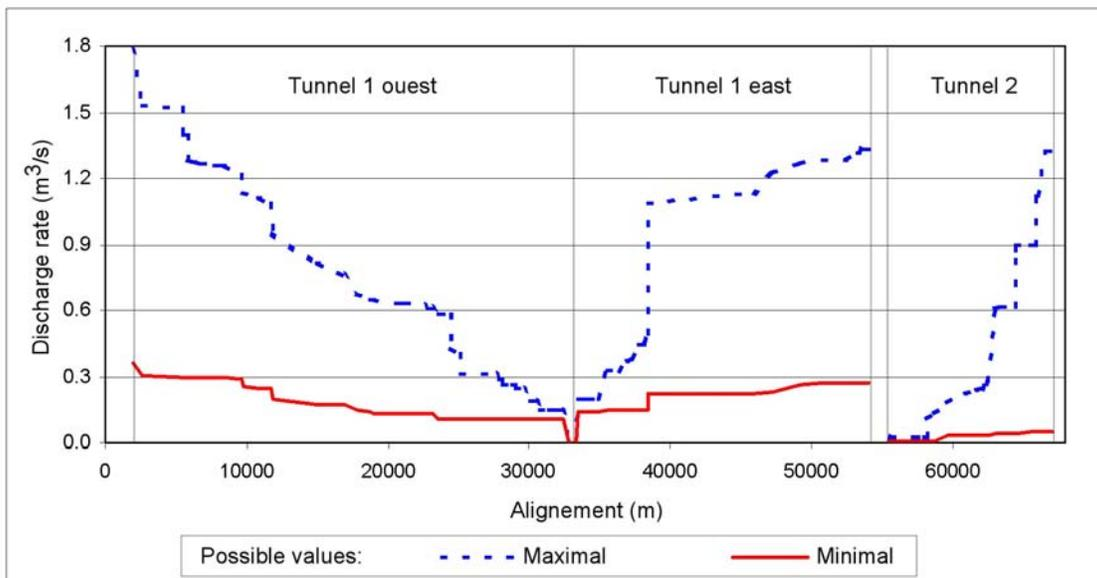
Fig. 2. Prediction of discharge-rates at the tunnel entrances of a 65 km long railway line in the Alps.
