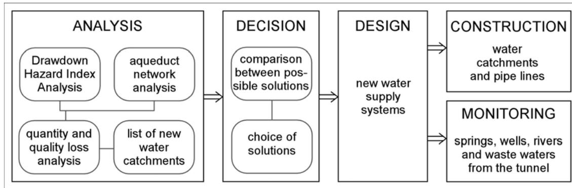
Fig. 4. Flow chart of water-supply compensation study to be performed in case of groundwater drawdown after tunnel excavation.
