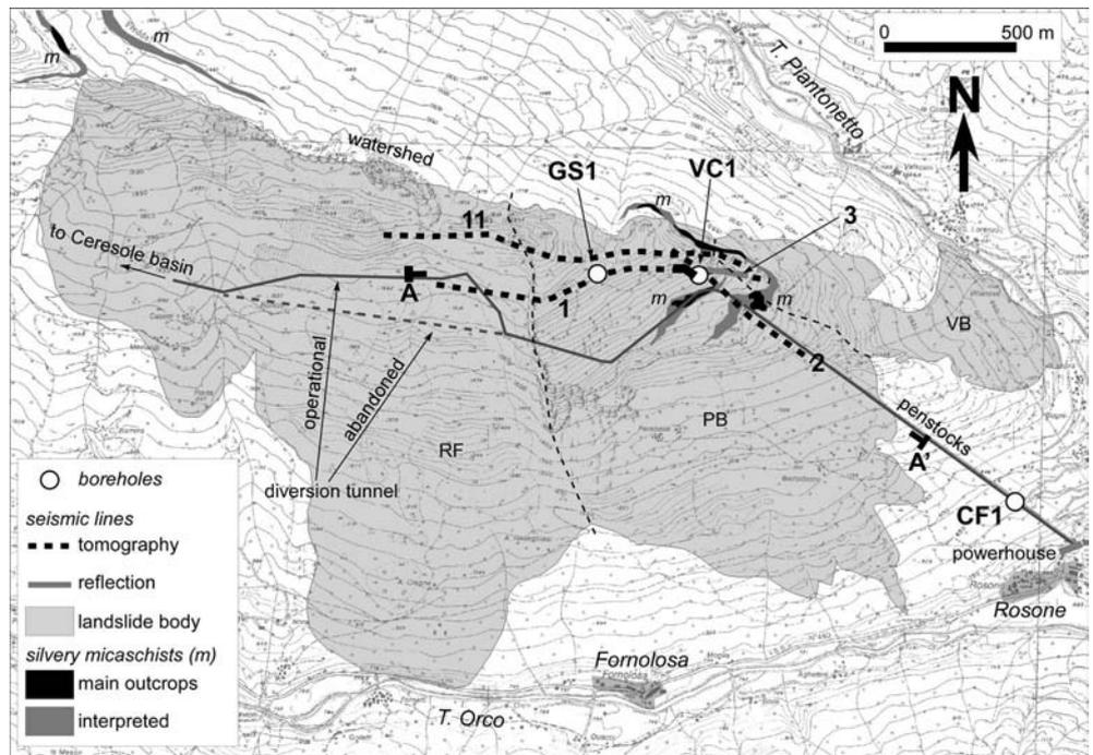
FIG. 2 - Synthetic map of the Rosone landslide area. The position of the IRIDE hydro-power plant and of the new investigations is indicated. RF: Ronchi-Fontane Fredde sector; PB: Perbella-Bertodasco sector; VB: Villanova-Buriat sector.
