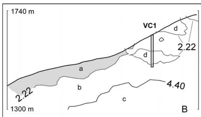
FIG. 7 - A: seismic tomography nr. 2 ( $V_p$ , km/s); B: simplified interpretative cross section. a: landslide; b: fractured rock mass; c: sound rock mass; d: low- $V_p$  basement (lithological and/or textural changes).
