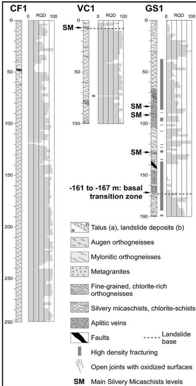
FIG. 5 - Synthetic borehole & RQD logs. Notice the discontinuous RQD in GS1, high RQD values above -163 m being related to competent rock slabs within the landslide. VC1 starts within the landslide and rapidly reaches a fairly sound basement, even though open fractures are recorded. CF1 is located outside the zone affected by movements.
